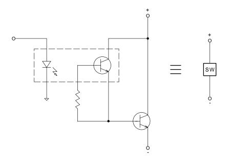
Figure 5.3 Isolated Loop Current Switch
