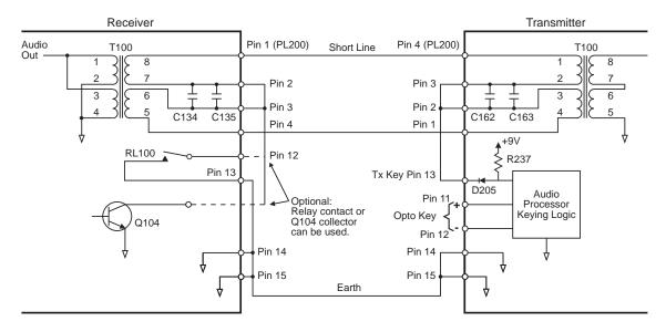
Figure 5.1 DC Loop Keying With Common Earth
